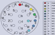
PWR+ PWR-N/C 00000000000 S: N/C 0000000000 RS-232-2 TXD RS-232-3 TXD RS-232-2 RXD RS-232-3 RXD N/C N/C N/C N/C N/C N/C
